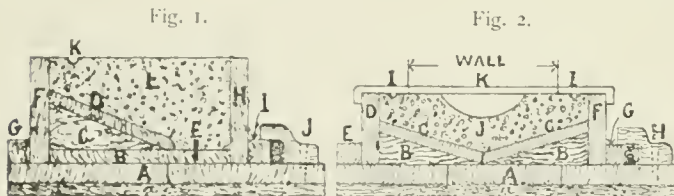
NO. 202.—FIG. 1.—SECTION OF MOULD FOR CASTING SILLS. FIG. 2.—SECTION OF MOULD FOR CASTING COPING.
